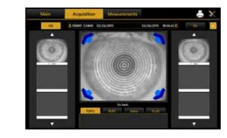
Acquisition The CA-800 is easy to use. Visual signals support fast and easy alignment and focusing on the patients eye. The CA-800 has a Right and Left eye detection and prevents incorrect savings in Right / Left eye measurements. The automated best image selection mode in the software of the CA-800 decides the best focused position and automatically acquires the image. Acquistions can be made for topography, pupillometry and real time fluorescein imaging.
